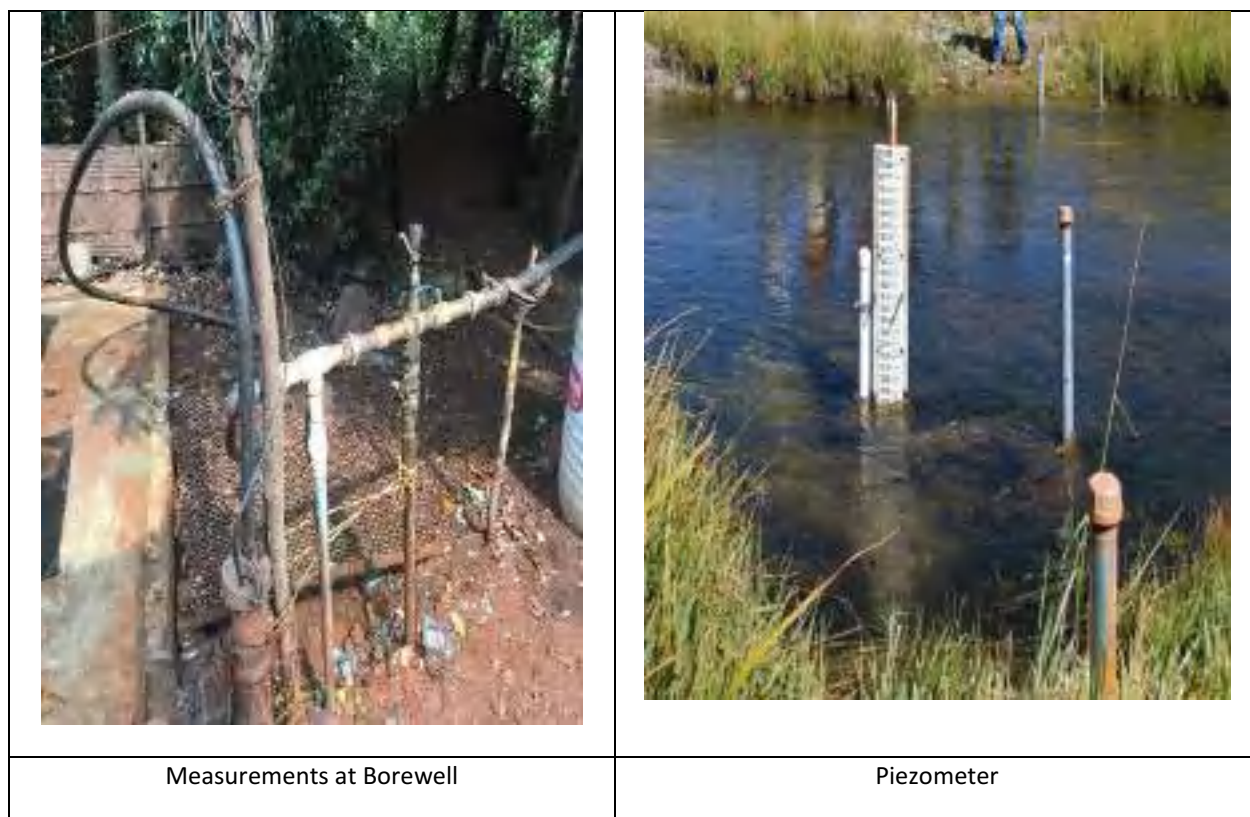
Picture 2: Picture taken during measurements at bore well and picture of Piezometer
